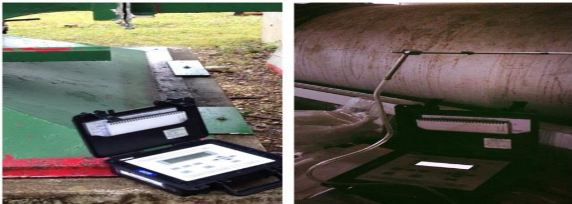
Figure 6.4. Transducers usage through the ducting
